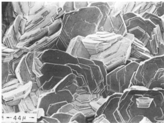
Fig. 11. Zinc deposited at 40° C and 200 mA cm -2 from Ni-free electrolyte. Electrolysis conditions: 0.5 N H 2 SO 4 ; 50 g l -1 Zn 2+ .
