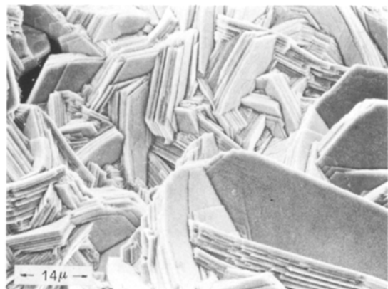
Fig. 10. Zinc deposited at 200 \text{ mA cm}^{-2} current density from Ni-free electrolyte. Electrolysis conditions: 0.5 N H_2SO_4 ; 50 \text{ g l}^{-1} Zn^{2+} ; 25° C.
